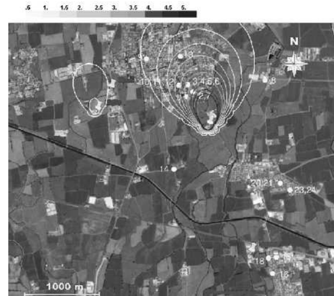
Fig. 5. Map of the ground peak odour concentration values on the 27th August 2008, between 7am and 8am.
